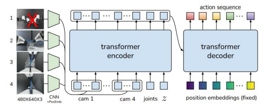
Conditional Variational Autoencoder (CVAE) structure (encoder-decoder), we are training transformer encoder, decoder's attention weights.
